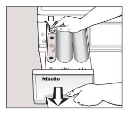
Pull out the detergent drawer as far as it will go. Press the red release lever down and pull the drawer out of the machine.
